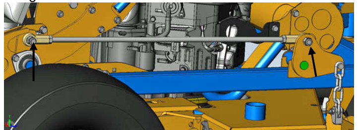
First ensure Deck Lift Rod is 29" from center to center of the ball ends
